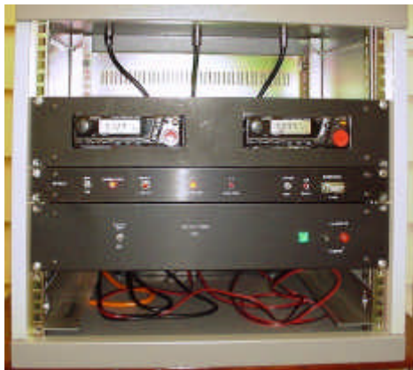
GB3DB Radios, CUL Logic and PSU in 19" Cabinet – almost complete, but working !
